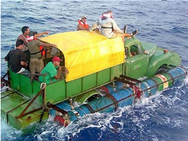
Twelve Cuban migrants were caught attempting to get to the US in a truck they had turned into a boat. They converted a 1951 Chevy pickup and used empty 55-gallon drums to keep it afloat. They attached a propeller to the drive shaft, giving the craft a top speed of just 8mph. A US Customs aircraft spotted the truck as the Cubans crossed the Florida Straits.
