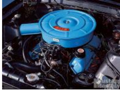
The base V-8 during the Mustang's first five months was the 260-2V with Light Blue valve covers and air cleaner. This is not the darker Ford Corporate Blue that came in '66. The air-cleaner snorkel on this engine should be black.
