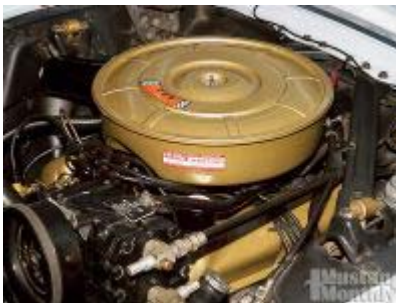
The base V-8 for August '64 and beyond was the 289-2V with gold valve covers and air cleaner. Identical in appearance was the Challenger V-8-the 225-horse 289-4V engine with higher compression. Black, heads, and intake were black. Some Canadian-delivered Mustangs received red valve covers and air cleaner. No one has been able to determine why.
