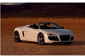
The GT Spyder is 10 mm lower than the R8 V10, and the suspension has a stiffer calibration. XYZ ventilated and cross-drilled rotors provide stopping power, with 19inch wheels at all four corners. Visual cues on the GT Spyder include a larger rear diffuser, front splitter and a fixed rear spoiler. The interior is black—period. Accent stitching can be ordered in gray or red, with Alcantara flatbottomed steering wheel, and parking brake, and seat insert trim... Saab Heritage Saved. De-'GMC's' spite
