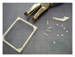
"Cut a few pieces of styrene rod to length. I am using .062 rod cut to 10mm. Using a hole punch cut out few disks that will act as the bearing plates."
